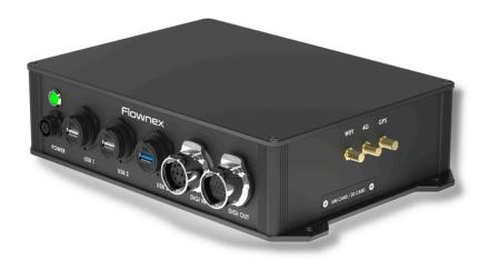
Flownex Edge, designed as an AI ready, fanless embedded computing solution with robust antivibration and anti-shock protection, finds its ideal application as an onboard unit within the transit sector.
